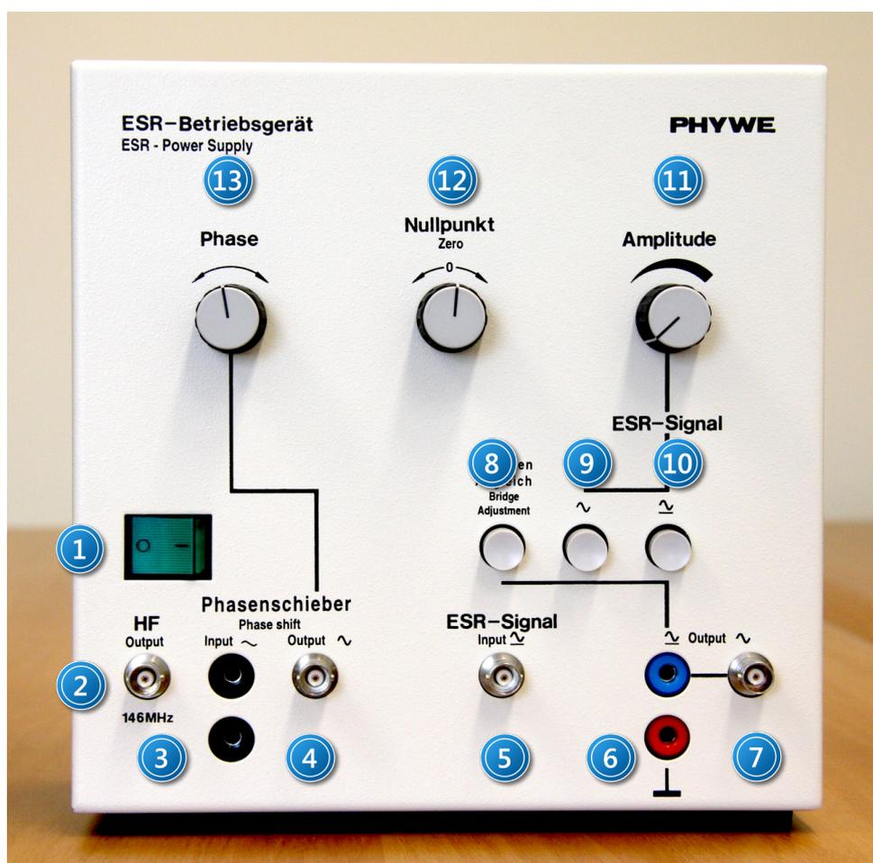
*Picture 5, Front panel of the EPR power supply: 1 – power switch; 2 – high-frequency output; 3 – 6V/50Hz internal phase shift output; 4 – phase shifter output; 5 – EPR resonator signal input; 6 – output to the digital meter; 7 – output to the oscilloscope; 8 – bridge balance check button; 9 – button to select oscilloscope signal only; 10 – button to select signal for the oscilloscope and meter; 11 – gain dial; 12 – zero dial; 13 – phase dial.*
