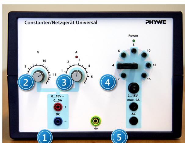
Picture 4. Universal power supply front panel: 1 – output voltage; 2 – voltage dial; 3 – current dial; 4 – AC voltage selection; 5 – AC voltage output.
