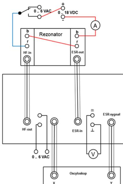
*Figure 2. Circuit diagram of components to measure EPR resonance: 1 – resonance cavity; 2 – EPR power supply; 3 – universal power supply; 4 – dual-channel oscilloscope; 5, 6 – digital multimeters.*
