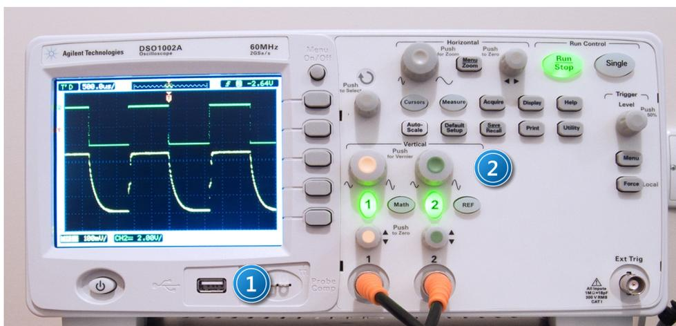
Picture 6. Oscilloscope front panel: 1 – USB slot; 2 – save/read data button.
