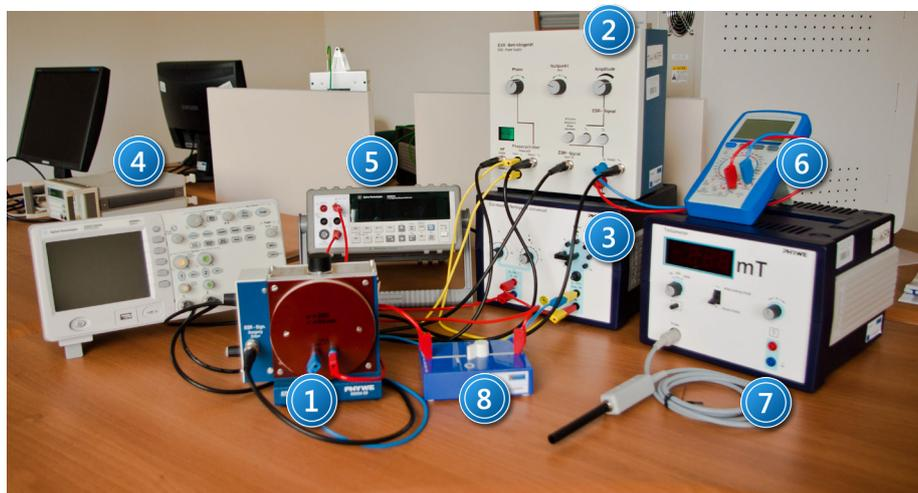
*Picture 1. Experimental setup for measuring EPR absorption lines: 1 – EPR resonance cavity; 2 – EPR power supply; 3 – universal power supply; 4 – dual-channel oscilloscope; 5 – digital multimeter (ammeter); 6 – digital multimeter (voltmeter); 7 - teslameter; 8 – switch.*
