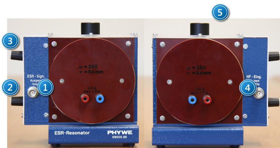
Picture 3. Left and right view of the EPR resonance cavity: 1 – EPR signal output; 2 – capacitance dial *C*; 3 – resistance dial *R*; 4 – high-frequency input; 5 – place for the sample.
