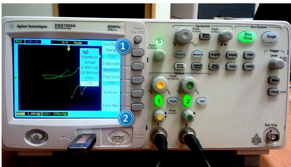
Picture 7. Write/read menu on the oscilloscope front panel: 1 – data type selection button; 2 – memory manager button.
